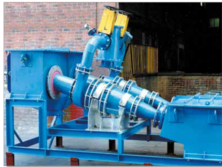
A completely assembled Multotec Dense Medium Cyclone Distributor, awaiting shipping to a Russian diamond operation.
