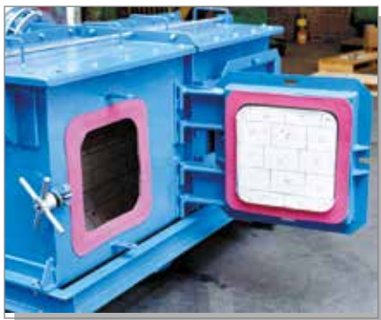
A completely assembled Multotec Dense Medium Cyclone Distributor, awaiting shipping to a Russian diamond operation.
